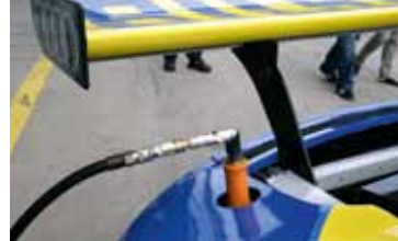
A new supply coupling for the pneumatic air-jack numbers among the changes
