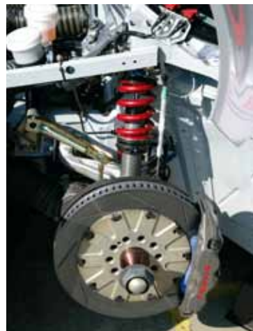
The ceramic braking system has been replaced by a steel counterpart
