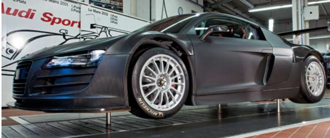
The three-point air-jack is designed for pit stops in racing
