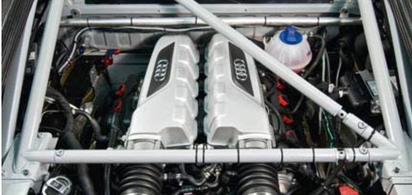
The 5.2 litre engine is located longitudinally in front of the rear axle
