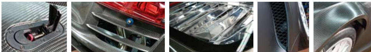
The bodywork preserves the fascinating appearance of the production car, but is made mainly of carbon fibre
